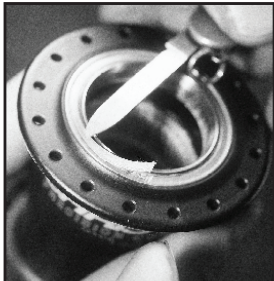
Figure 12 - remove snap ring
