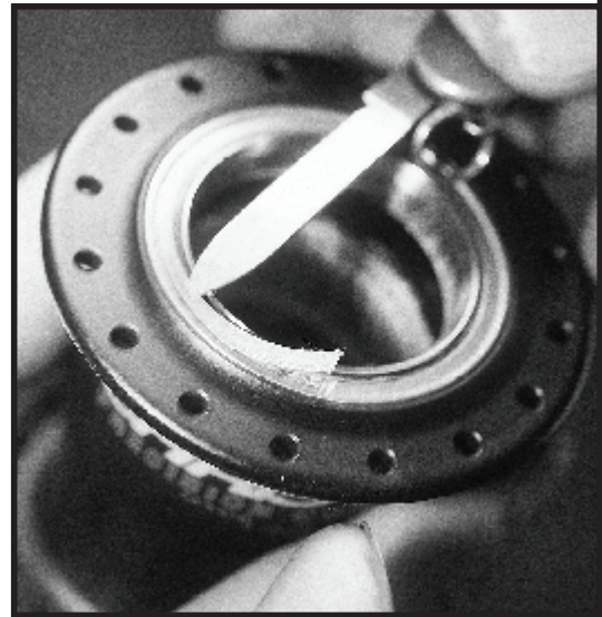
Figure 26 - remove snap ring
