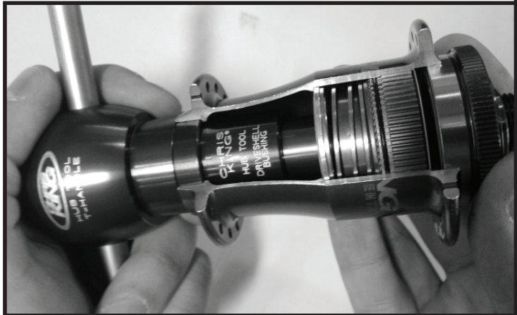
Figure 32 - press drive side bearing
